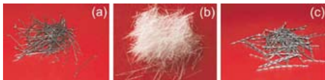
Fig. 2 - Fibre impiegate: (a) acciaio, (b) PVA e (c) PPHT.
