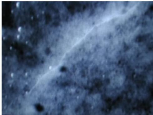
**Fig. 10 – White material filling the pre-existing cracks.**
