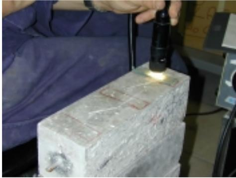
**Fig. 9 – Observation of the width-crack by optical microscope.**
