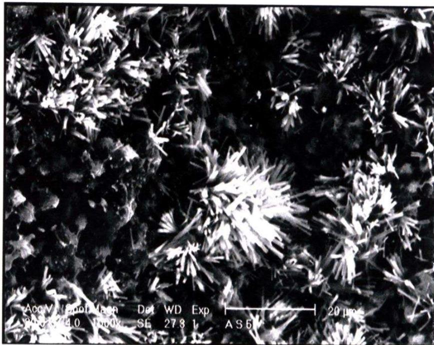
Figure 3 – Morphology of ettringite and/or thaumasite crystals grown into a crack formed by immersion in sulfate solution (2 days at 5°C) alternated with a drying period of 5 days at 40°C.
