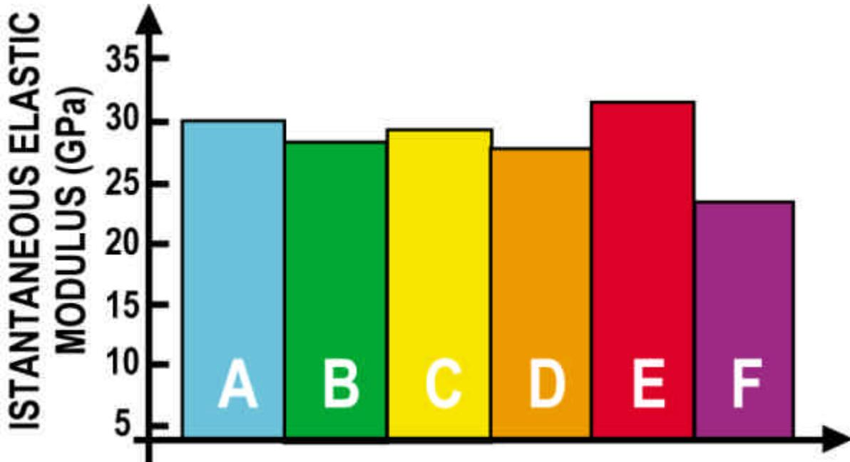
Figure 19 - 28-day elastic modulus for six shrinkage-compensating mortars.
