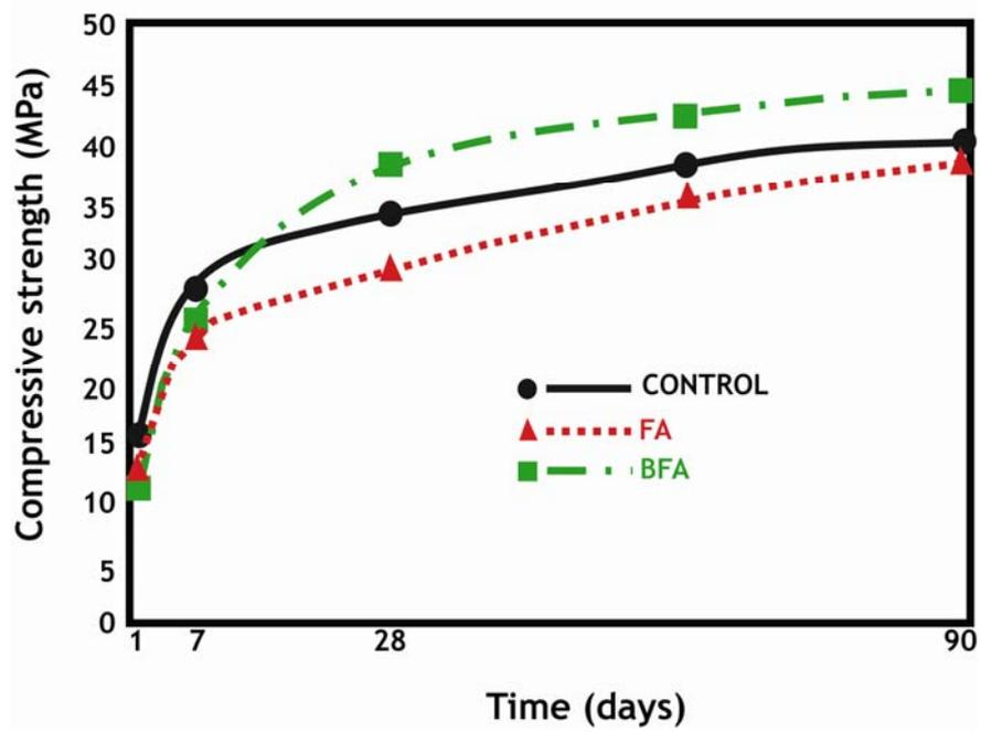
Figure 1 - Influence of FA or BFA mixtures on the compressive strength at 1, 7, 28, and 90 days.
