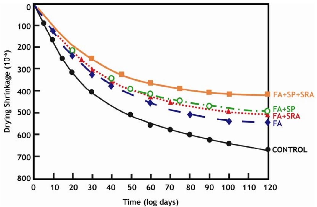
Fig. 2 – Unrestrained drying shrinkage of control and FA mixtures.
