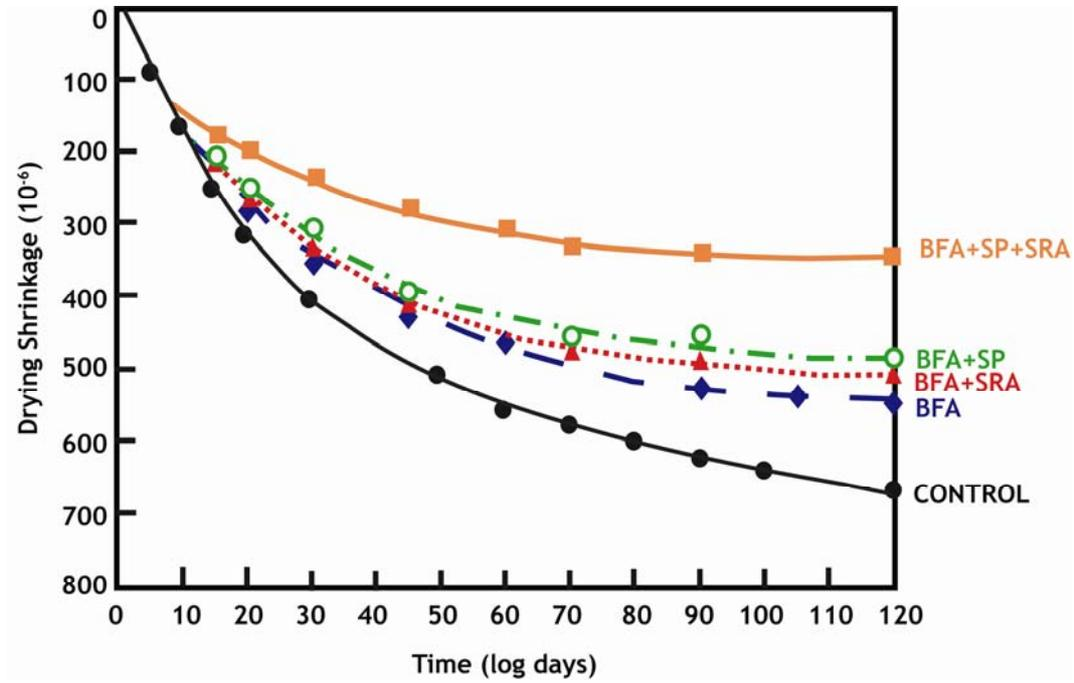
Fig. 3 - Unrestrained drying shrinkage of control and BFA mixtures.
