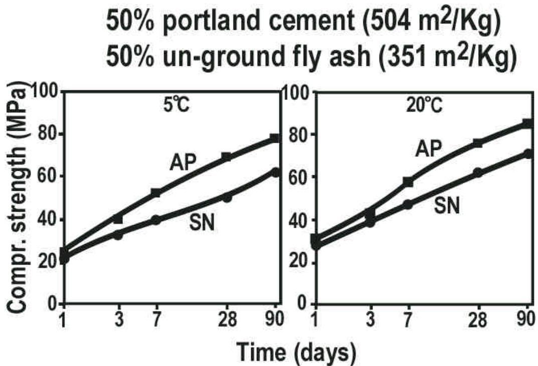
Fig. 4 - Influence of temperature and superplasticizer type on compressive strength versus time (cement C).
