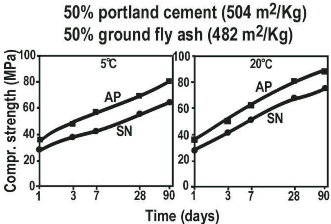
Fig. 5 - Influence of temperature and superplasticizer type on compressive strength versus time (cement D).
