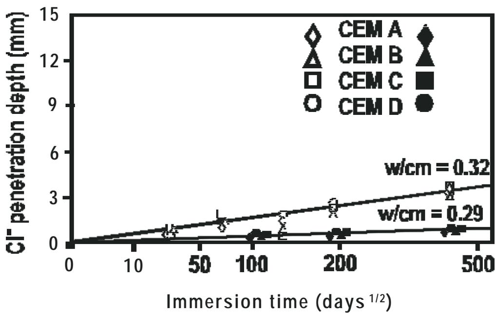
Fig. 7 - Chloride penetration in HVFA concretes as a function as the cement fineness (Table 2) and superplasticizer type (SN or AP).
