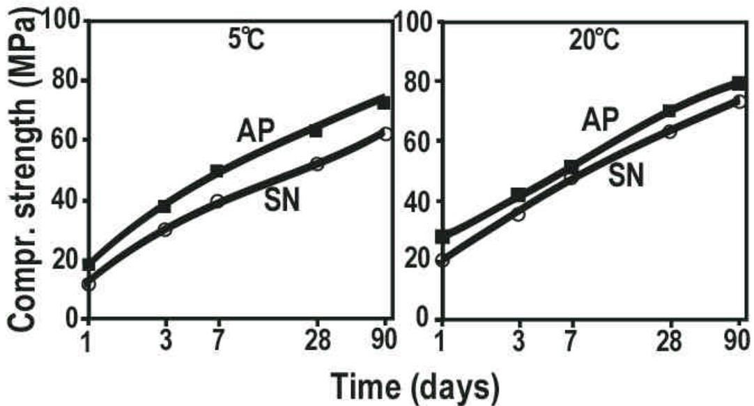
Fig. 2 - Influence of temperature and superplasticizer type on compressive strength versus time (cement A).
