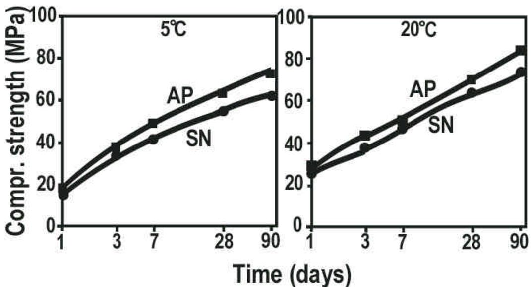
Fig. 3 - Influence of temperature and superplasticizer type on compressive strength versus time (cement B).
