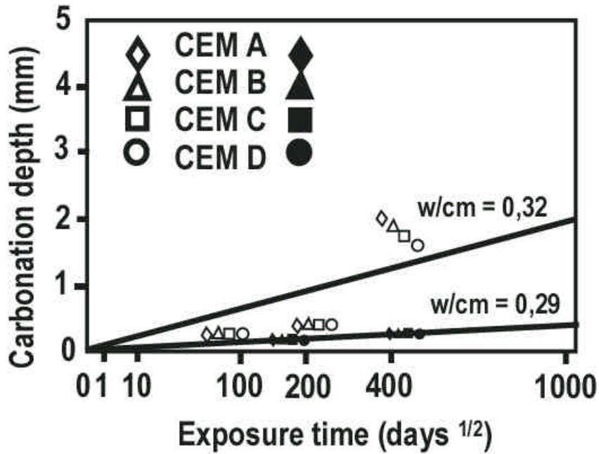
Fig. 6 - Carbonation of HVFA concretes as a function of cement fineness (Table 2) and superplasticizer type (SN or AP).
