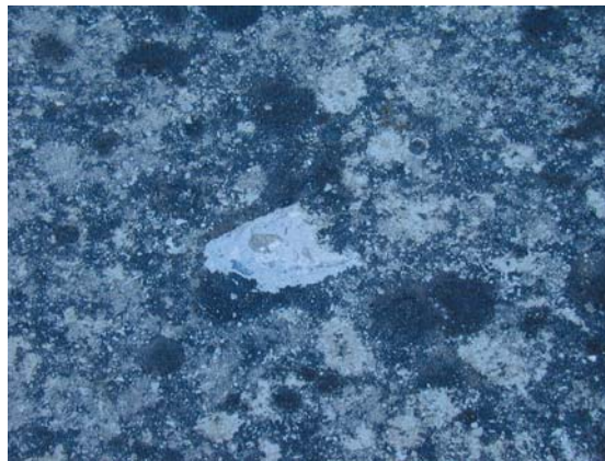
ig. 13.6 – Microscopic view of mass on the dark surface of the building in ig. 13.5
