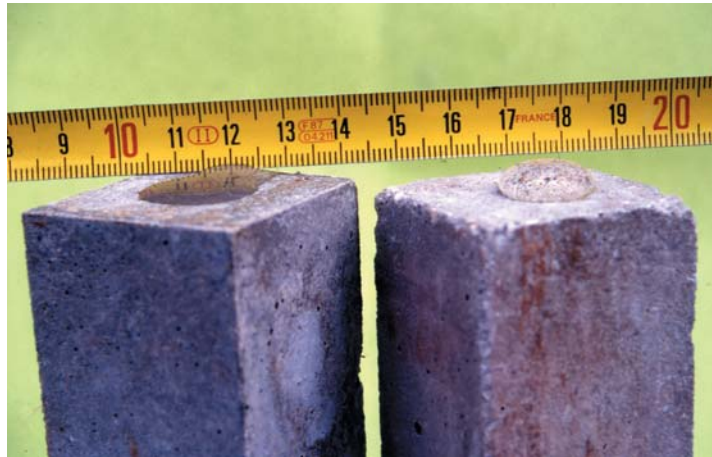
ig. 13.4 – A drop of water on plain concrete specimen (left) or on concrete specimen after treatment with silane
